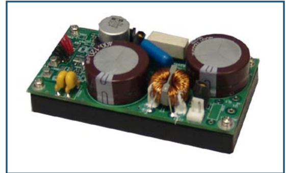
Image displays unit with EMI filter & control board
